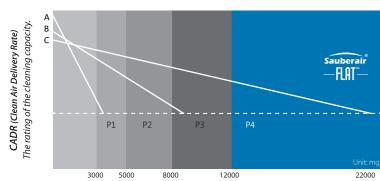
CCM-Cumulate Clean Mass (=Dust holding Capacity= Filter's lifespan)
